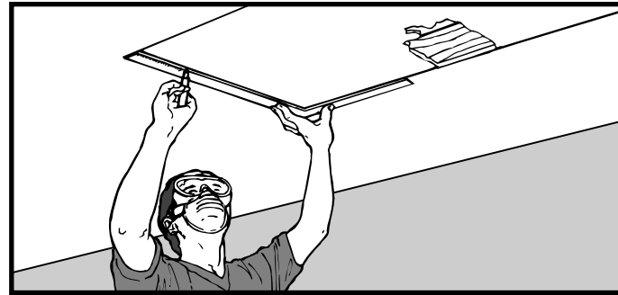
Figure 7. Draw a rectangle the size of the rough opening.
